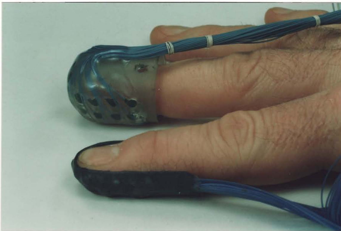
FIGURE 43: Top: Inactive tactile display prototype with 41 dummy taxels embedded in a flexible latex substrate (Photo. GC170595A-08). Bottom: The flexible tactile display is much smaller and easily conformable to a wide variety of finger size, as compared to the larger and inflexible Phase-I device (Photo. GC160595A-16).
