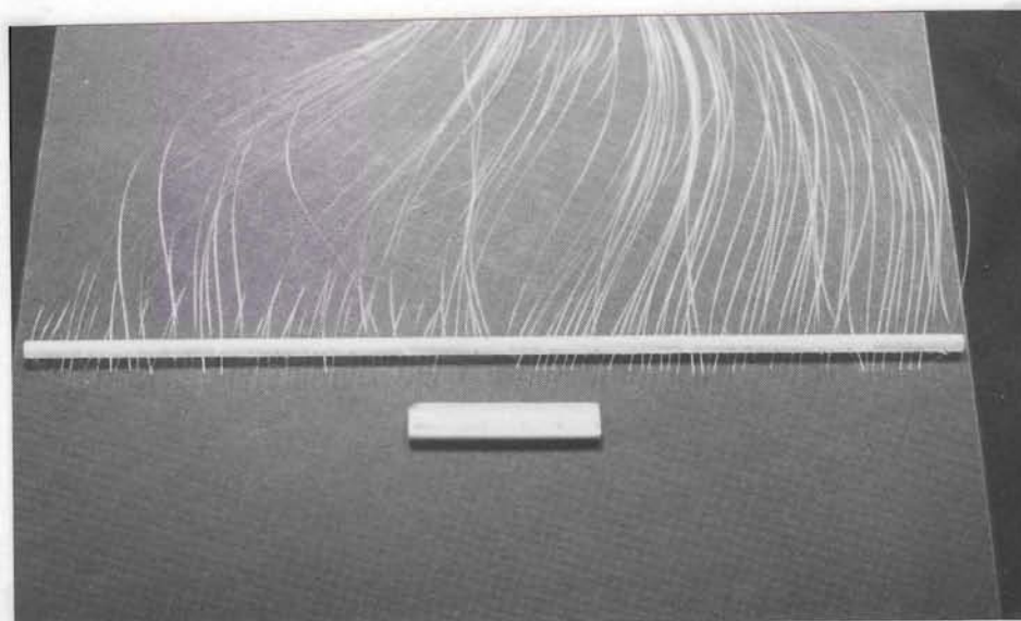
FIGURE 10: Optical sensor fibers (101 total) threaded through the linear fiber substrate. Fibers have been potted into their holes, but not fully trimmed or encapsulated into the substrate core.
