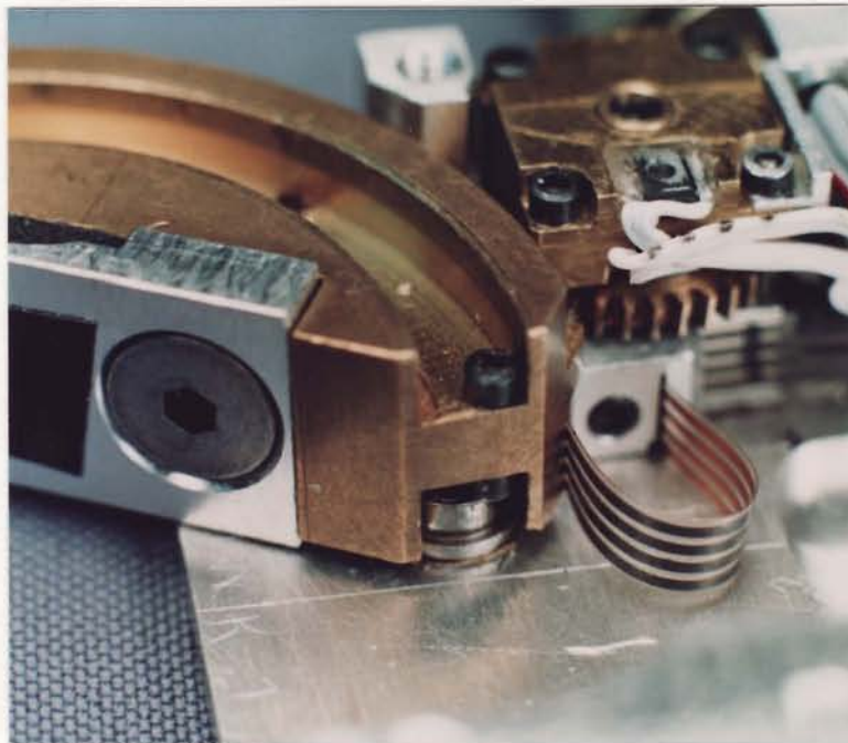
FIGURE 2.4-5: The safety of the glove controller was ensured by the presence of hard mechanical stops to limit joint motion. Failure-proof structural body stops were used to limit the extension motion of the virtual-hinge joints (top-right) and the lateral motion range of the pin-hinge (center-left), whereas semi-hard stops to block the bearing channels in the slider were used to limit finger flexure motions (note screw heads in bottom right photograph). Failure of the latter stops was considered tolerable, as self-disassembly of the hinge would quickly follow.
