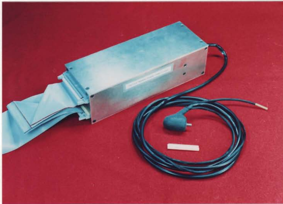
FIGURE 4.2-1: Compact 48-channel tactile signal conditioner fabricated for this program (top) coupled to a 37-channel optical tactile sensor (center). The unit weighed 0.9 kg, and measured 90 mm x 70 mm x 250 mm.
